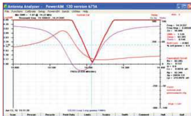
FIGURE 4: Measurements of SWR, Z magnitude and Theta of the finished loop. Compare the SWR with that predicted in Figure 2.
