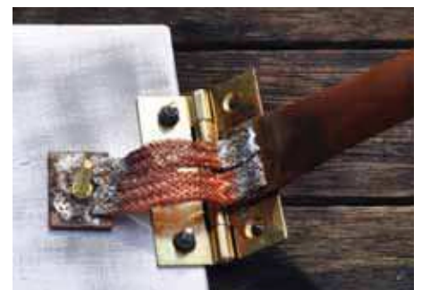
PHOTO 2: Detail of the capacitor hinge.
