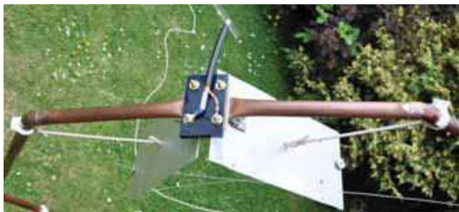
PHOTO 3: Construction of the variable capacitor with an additional parallel fixed lower frequency capacitor made from a short length of RG213 (see text).
